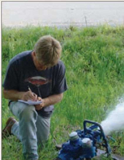
Good water loss accountability begins by verifying the accuracy of master meters. Here the author records results of one such test.
