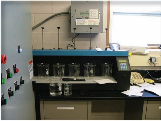
Surface water treatment plants should have jar testing equipment similar to this at the Kickapoo Plant to help optimize chemical usage. This is especially important with changes in raw water turbidity or temperature.
