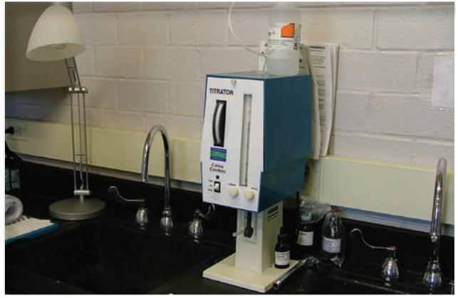
Amperometric titrators similar to this are used in surface water plants to accurately measure chlorine residuals. It is very important when feeding ammonia to form combined chlorine that accurate chlorine residual test results are obtained when trying to reach the proper ammonia to chlorine ratio.
