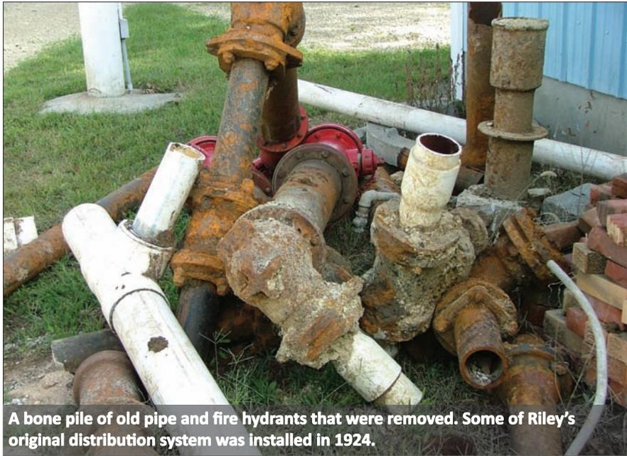
A bone pile of old pipe and fire hydrants that were removed. Some of Riley’s original distribution system was installed in 1924.
