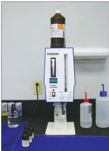
**Amperometric titrators such as the one shown here can distinguish different types of chlorine residuals (free, combined, monochloramine, and total).**
