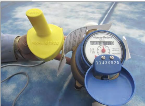
**Dan Dehn is holding a new radio meter similar to those installed in the district. Installing these meters has allowed district staff to read the meters monthly and should provide more accurate information. This information along with the replacement of the problem line should result in less water loss.**
