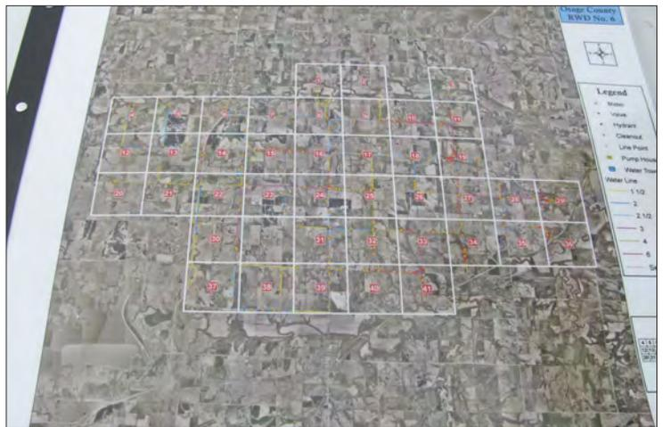
**This digital map was produced for the district by KRWA. The map was available prior to this project and proved valuable to the district when determining quantities at the end of the project. Rather than paying the contractor plan quantities, the maps were used to confirm the measurements taken by the inspector in the field. The up-to-date digital maps saved the district money when it was determined that actual footage was less than plan quantities.**
