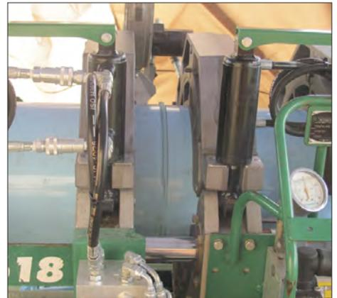
These four photos show the pipe fusing sequence: Top left photo shows an employee in the process of evening up the pipe ends with a facing tool. Note the facing tool in the next photo, top right. Next photo lower left, an employee has picked up the hot iron which will be inserted between the pipe ends, heating it sufficiently to form a bead. The last photo, lower right, shows the two pipe ends fused together.
