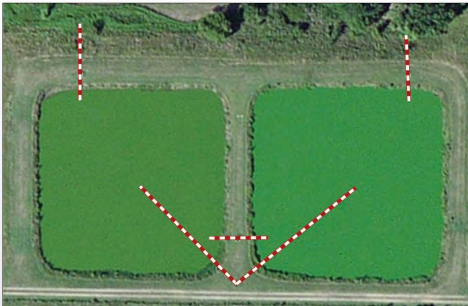
**Diagram A: Wastewater lagoons designed and constructed in the mid-1960's had the influent pipes placed to the center of the cells, and had the transfer pipes from cell to cell located in the center of the dikes. These discharging systems may even have discharge structures from each cell in a two-cell system.**
