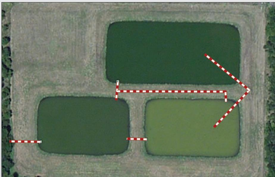
**Diagram B: Due to the design, some older 3-cell systems also have piping to the middle of the cells.**
