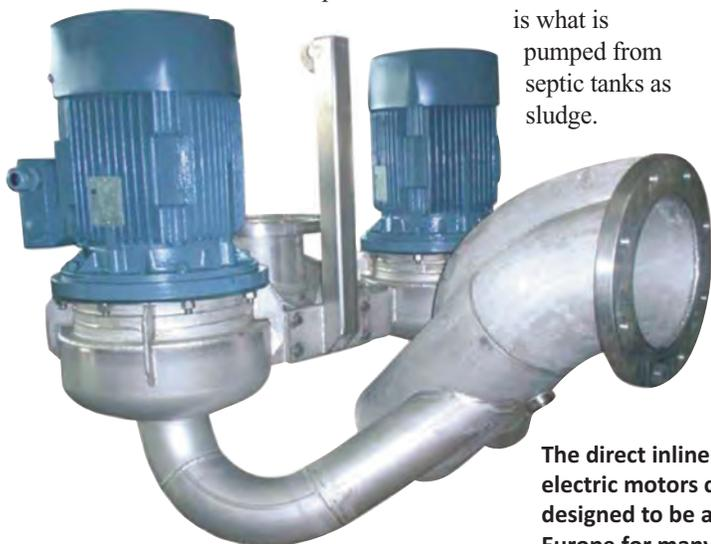
**The direct inline pumping technology featured in this article consists of two electric motors connected by a hydraulic body, the shape of which is specifically designed to be able to receive effluent directly. The technology has been used in Europe for many years and is advertised to eliminate clogs on its own.**
