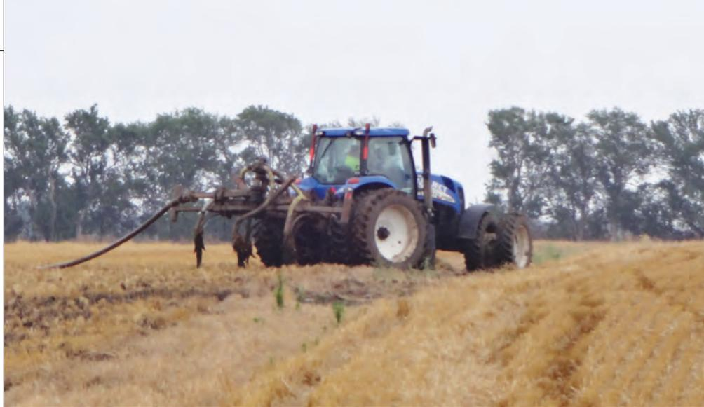
This tractor with injection system is used to "knife" the sludge under the ground surface. While surface application is allowed, injecting or disking is a better option as it reduces the possibility of runoff and odor complaints.
