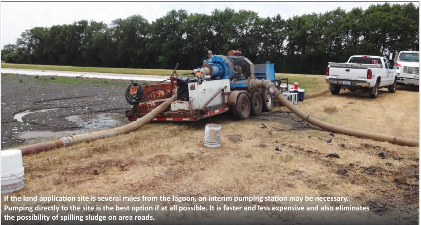
If the land application site is several miles from the lagoon, an interim pumping station may be necessary. Pumping directly to the site is the best option if at all possible. It is faster and less expensive and also eliminates the possibility of spilling sludge on area roads.
