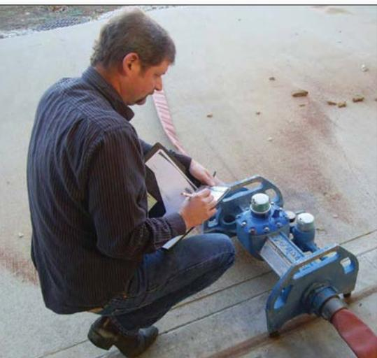
In this test at Suburban Water Company, the flow rate will be variable as this section of the system is supplied directly by pressure from the Board of Public Utilities, Kansas City, Kansas. This KRWA test meter is certified up to 400 gpm. KRWA also has non-intrusive meters to check larger meters operating at much higher flow rates.
