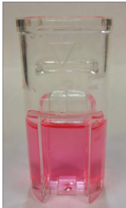
The plastic vial is only used in High Range. The vial is filled to the 5-ml mark. Also note the raised triangle near the top of the vial. This triangle should be facing away from the keypad before covering with the instrument cap and taking readings.
