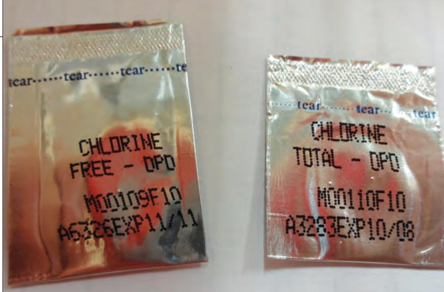
This photo shows the foil powder pillow packets for both free (left) and total (right) chlorine. The packet expiration dates can be found in the last line. The free packet on the left expired in November 2011 (EXP 11/11). The total packet on the right expired in October 2008 (EXP 10/08). Operators should check their supply of powder pillows and replace them if expired.
