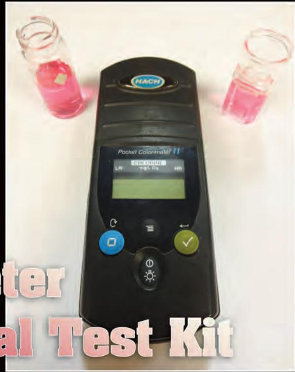
The above photo shows the Hach Pocket Colorimeter II with glass vial on the left and plastic vial on the right.
