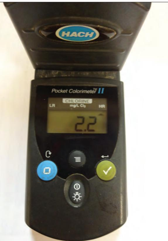
Note the reading of 2.2 mg/L is taken in High Range (note arrowhead below HR). Consequently, the readout would not be flashing. However if this reading were taken in Low Range, it would be flashing, indicating the reading is 2.2 mg/L or higher and that it should be analyzed in High range.
