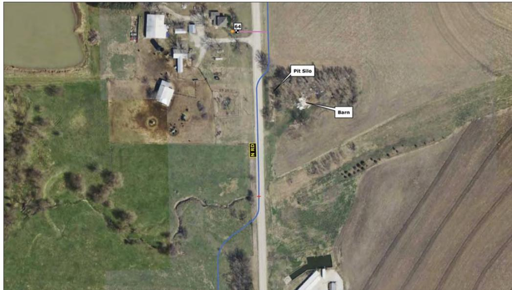
The graphic above shows a rural waterline entering the road and running north and south along the west edge of the road. The red X represents a GPS point that was collected by KRWA, at the location where the township road crew hit the waterline while replacing a drainage tube. The location of the waterline was not known prior to the damage.
