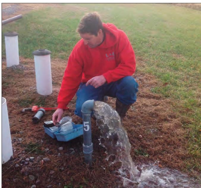
Superintendent Ellis checks chlorine residuals in flushed well water. Well No. 5 was flushed until no chlorine residual was detected.
