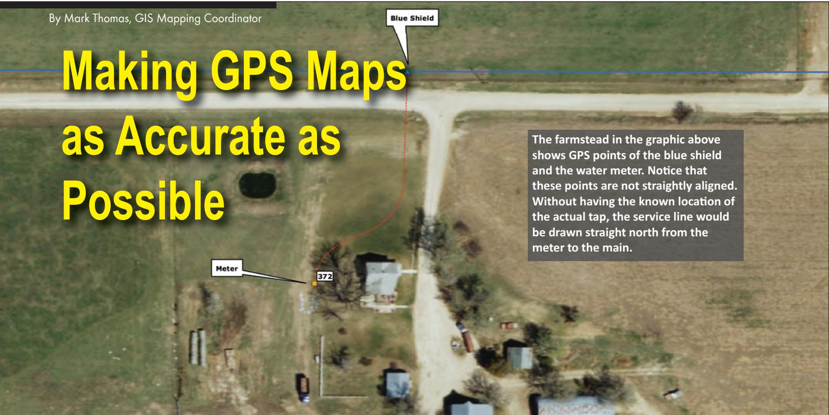
The farmstead in the graphic above shows GPS points of the blue shield and the water meter. Notice that these points are not straightly aligned. Without having the known location of the actual tap, the service line would be drawn straight north from the meter to the main.
