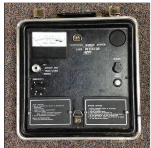
This locator is used by the RWD to locate the blue shields. A strap is attached to the metal loops shown on the top, turn it on, and wand it back and forth like a metal detector. The blue shield is found when the unit buzzes.
