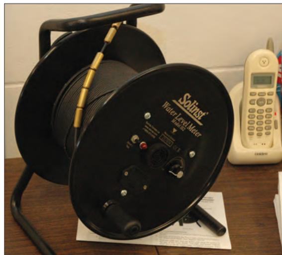
**This is a photo of a water level meter used to measure static and pumping levels in the wells. Measuring these levels is needed for calculating drawdown. Maintaining these records when a well is new and operating at optimum conditions provides valuable background information for later when the well is no longer operating at peak performance.**
