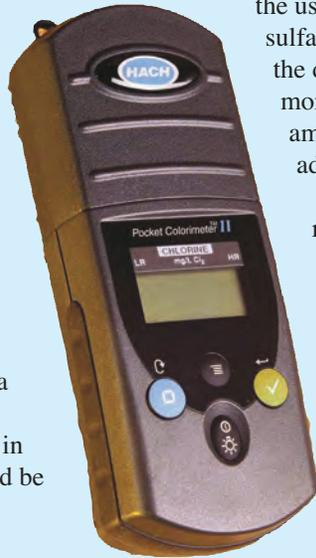
A hand-held DPD colorimetric tester such as this Hach unit with digital readout is one of the most commonly used monitoring devices in Kansas.
