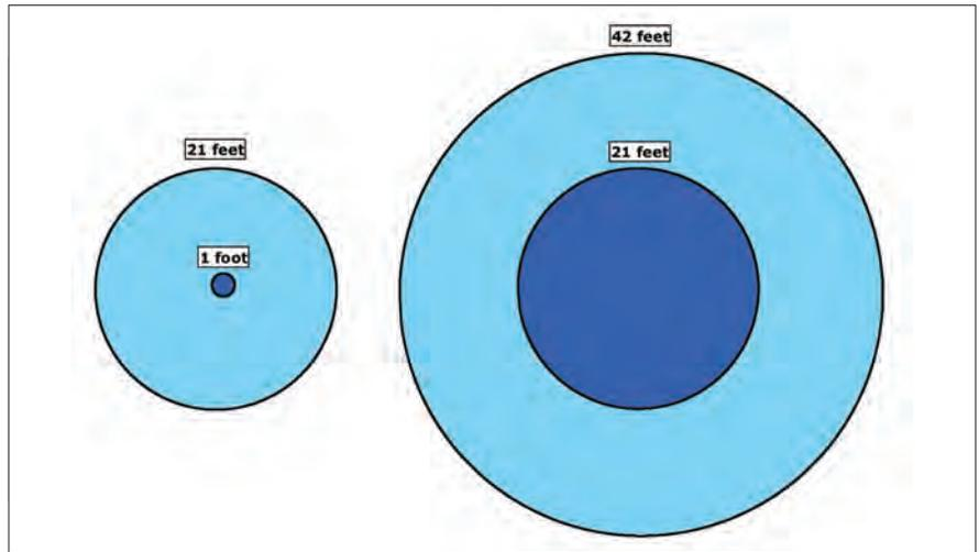
**These circles depict the degree of inaccuracy if someone were to collect a location with GPS on a smartphone. The circle to the right shows how the inaccuracy is compounded when that same point is located with a cell phone.**
