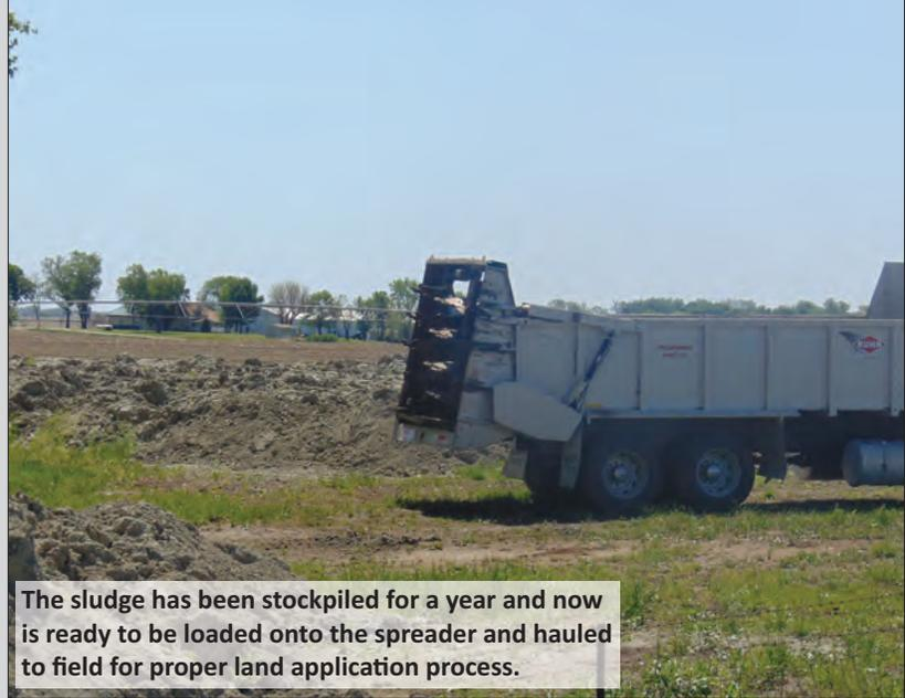
The sludge has been stockpiled for a year and now is ready to be loaded onto the spreader and hauled to field for proper land application process.
