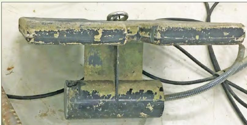
**This device is an ultrasound emitter. The large flat portion at the top provides the flotation for the device. The transducer hangs approximately six inches below the water surface. This particular device can be secured in place with nylon ropes and is tied to opposite sides of the Franklin RWD 6 settling pond.**
