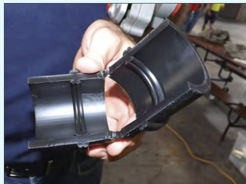
Cutaway of butt fusion
