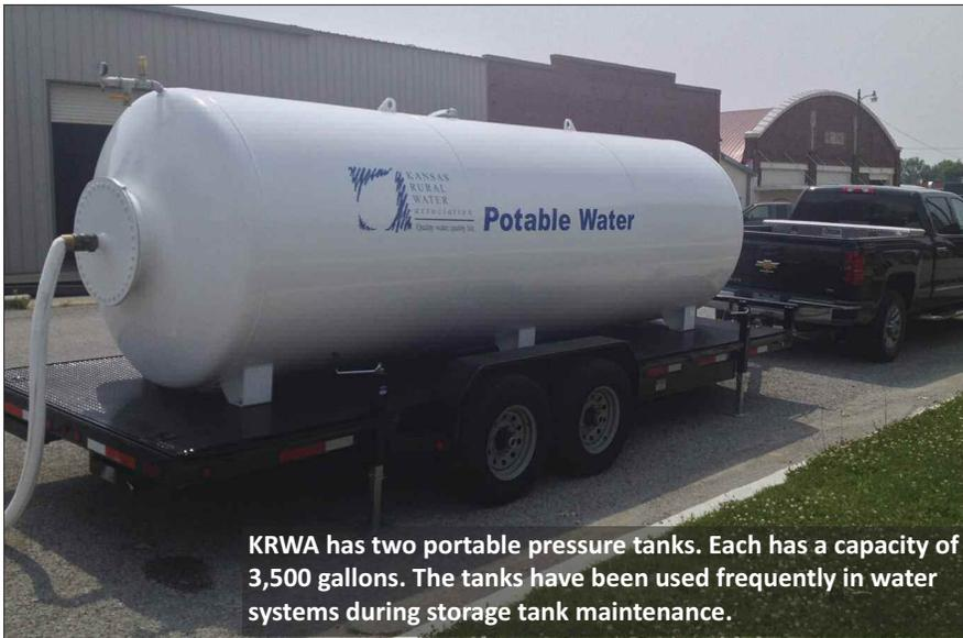
KRWA has two portable pressure tanks. Each has a capacity of 3,500 gallons. The tanks have been used frequently in water systems during storage tank maintenance.
