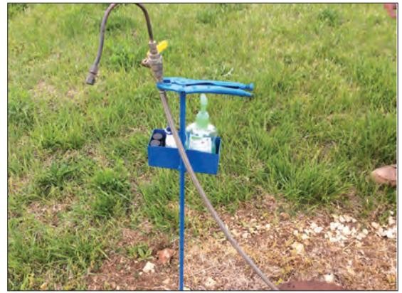
Butler RWD 3 Operator Jimmy Davis created this accessory storage and holding device to help collect samples using the GDW Sampler.
