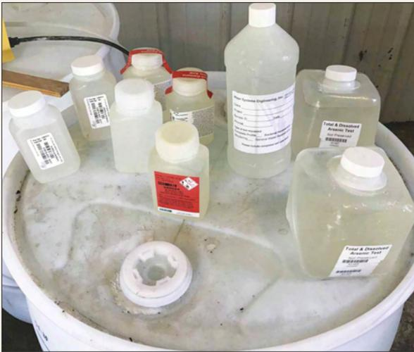
**It requires numerous containers for water samples for the various parameters for just one water sample at one location and one time.**
