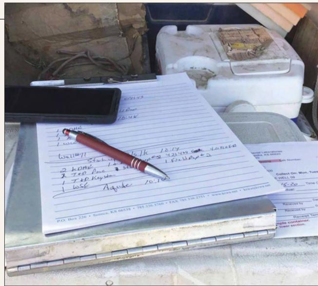
Notes logged on-site help ensure correct sampling location, sampling time, and each parameter.
