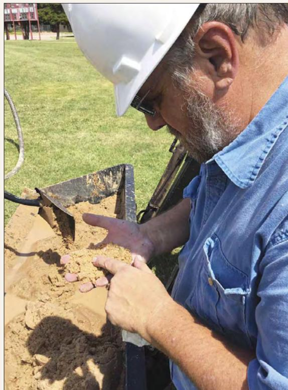
**Hydrogeologist Ned Marks of Terrane Resources, Stafford, Kansas, evaluates subsurface geology from a test hole for well water quality and water production purposes.**
