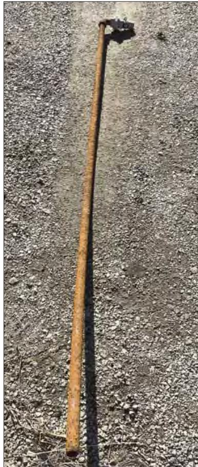
**This section of steel service line is very corroded due to soil conditions. It is from a small municipal water system in northeast Kansas.**
