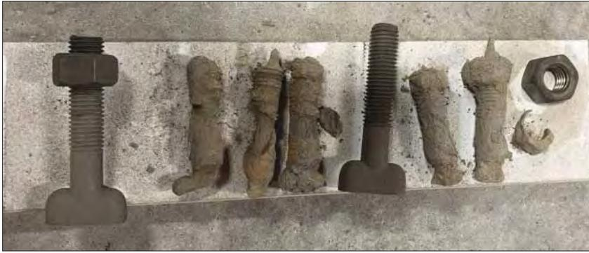
**These repair clamp bolts were very corroded after being in the ground for only three years in a small city in northeast Kansas.**
