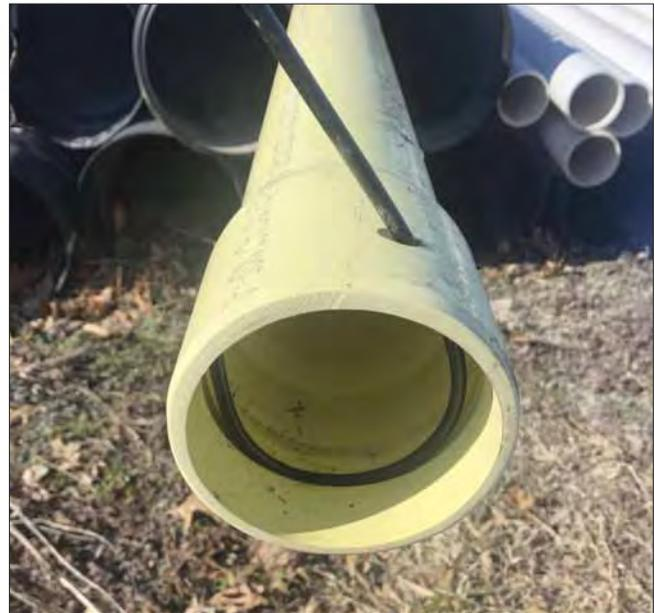
**The Yelomine pipe incorporates a locking self-restraining joint which has grooves that allow a spline to be inserted to create a restrained joint that locks the pipe and coupling together.**
