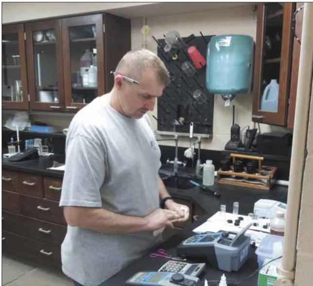
City of Garnett Water Treatment Plant Operator Jeff Mucklow, runs a chlorine residual test on a sample collected out of the clearwell.
