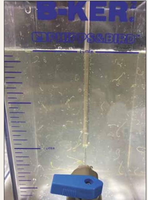
**Insoluble organics are shown as produced during a jar test dosed with 5 mg/L of Sodium Permanganate.**
