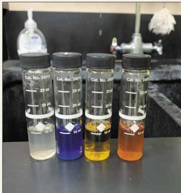
**This photo shows samples taken from a raw water source. The blue indicates high iron levels, and the deep orange is showing large amounts of manganese.**
