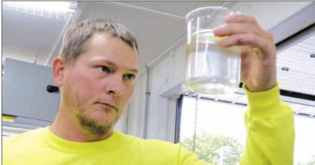
Wastewater operator for the city of Sabetha, and KRWA's first apprentice, Clint Bivens, inspects a sample pulled from the effluent of the city's activated sludge wastewater treatment plant.
