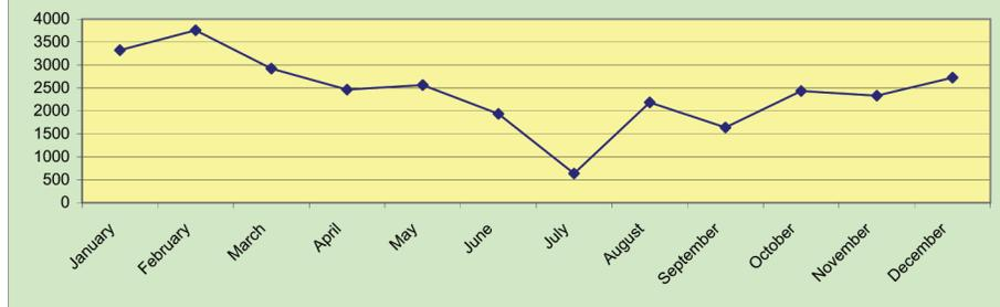
The above chart demonstrates part of the process that Kansas Rural Water Association completes when a utility requests a water loss survey. In the case of this city in Kansas, the “Unaccounted For Water” ranges from a low of 3.8% in July to 24% in February. These fluctuations indicate there are problems with meter reading or reporting rather than necessarily the loss being due to leakage.
