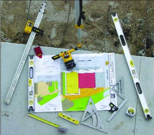
Shown in the picture are many "measuring sticks" used on KAN STEP projects. They include from left: transit grade stick, medium level, sight transit, torpedo level, square with angle-finder, architect's plan, swanson speed square, "T" square, tape measures and framing level.
