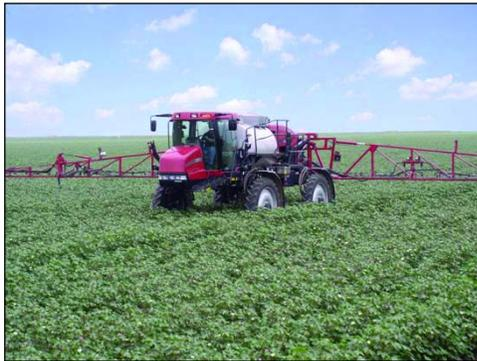
*A self propelled crop sprayer, pictured above, has the clearance with the high wheels and the speed to spray a lot of crop acreage in a day – or a lot of pipe.*
