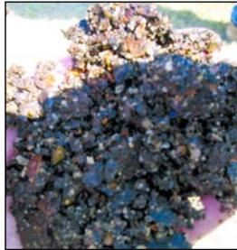
Weeks later, the operator informed me that the master meter stopped functioning. Inspecting this two-year-old meter, I found the bearings trashed and the turbine with extensive erosion to the turbine blades. This was all due to pumping sand. We installed another sand screen at the exit of the submersible well pump to protect both the meter and second screen in front of the chlorinator booster pump.
