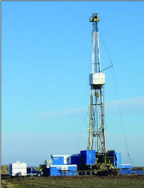
*This oil well drilling rig in Ness County was found making good progress on a warm December afternoon in 2004. Water is an important component of drilling fluid, which carries rock from the bottom of the borehole and seals the formations the drill bit encounters.*
