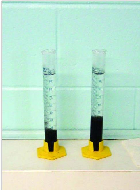
*These are pictures of graduated 100ml cylinders that the Sabetha city plant operator uses to do settleability samples from the center cone of the solids contact basins. The photo at left was taken immediately after the samples had been drawn. The operator lets the samples settle for 30 minutes and then determines the solids level for each basin. The photo on the right shows solids levels of 25% and 40%.*
