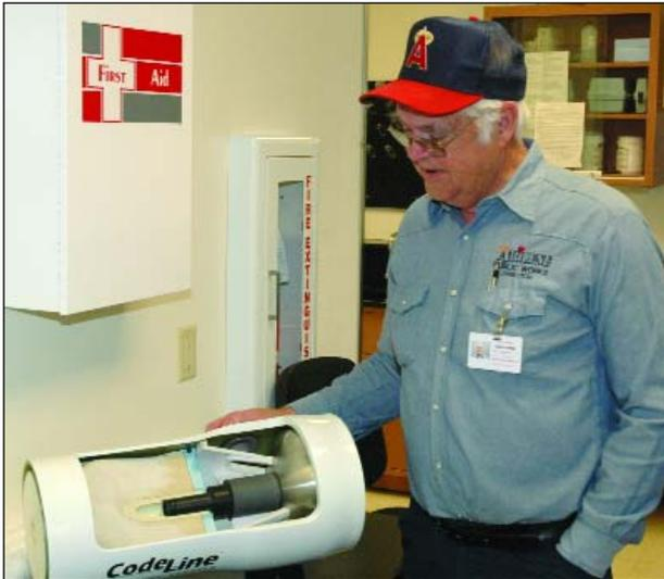
Cliff Gibbs describes the workings of the plant's RO tube units with the cutaway model on the table. The off-white semi-permeable membrane is seen at the left end of the model.
