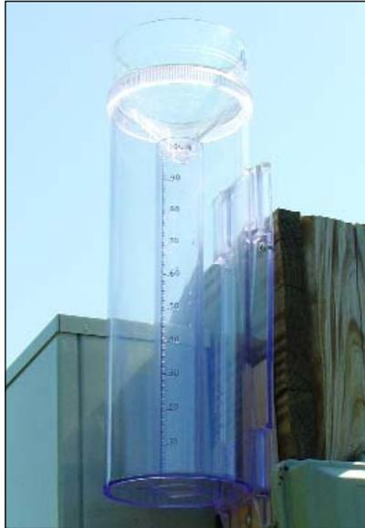
*A rain gauge, like this one available from K-State Extension's Weather Data Library, is the standard tool for measuring precipitation in the CoCoRaHS program. It measures precipitation in hundredths of inches and has a capacity of over 11 inches. It is very accurate, and is easy to mount on a flat-sided fence post.*
