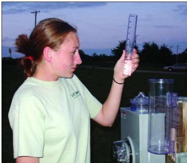
Reading the gauge is as simple as removing the small tube from the large tube and comparing the lowest level of the water's meniscus to the graduations on the tube.
