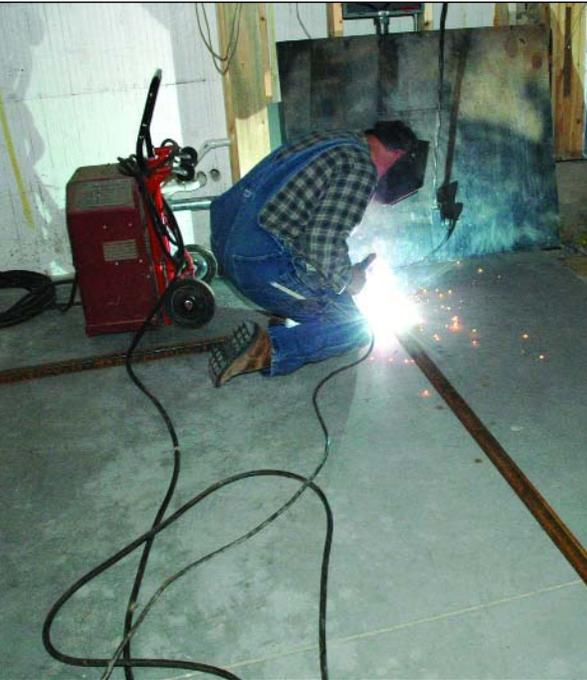
**Above:** Project Sparkplug Les Schneider is busy making sparks as he welds the steel tubing frame for the theater's behind the stage, moveable movie screen frame.
