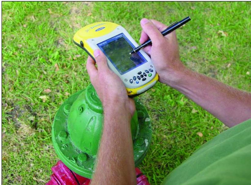
*Kansas Rural Water Association uses Trimble GeoXH™ handheld GPS data collectors for GPS mapping. The GeoXH is billed as Trimble's top-of-the-line solution for high accuracy GIS data collection. The handheld delivers the subfoot (30 cm) GPS accuracy required by water and wastewater services, electric and gas utilities and other applications where accurate positioning is crucial.*
