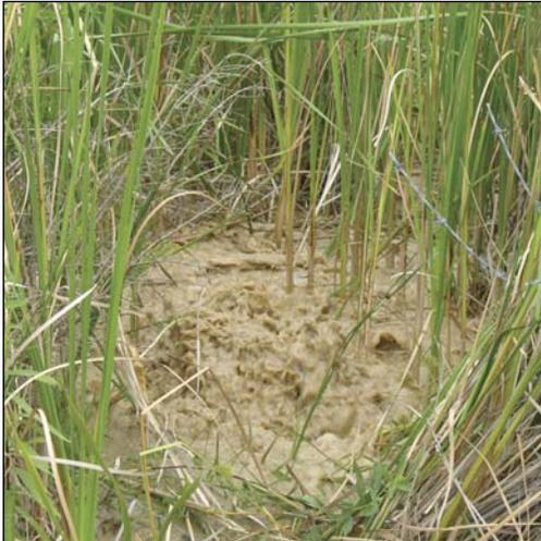
**Above:** An increase in line pressure can force a leak to the surface. On the water loss survey at De Soto, a mainline valve was fully opened increasing pressure from 25 to 76 psi. It brought the leak shown here to the surface.
