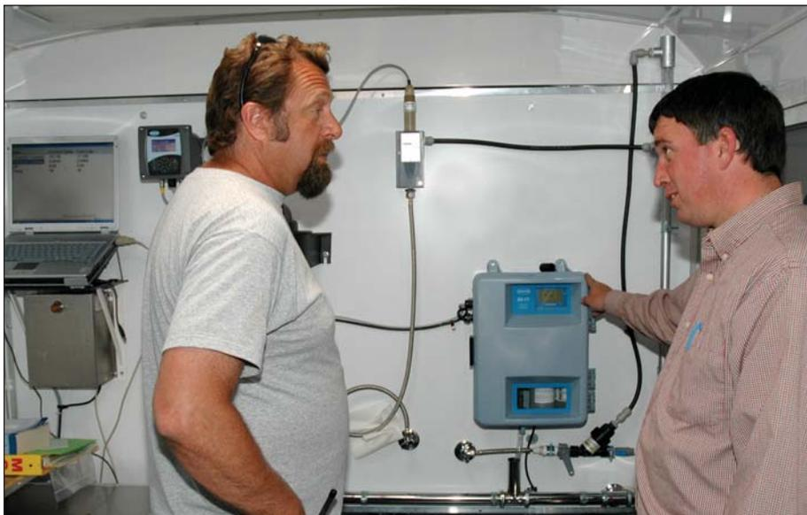
**Top:** A year ago KRWA Tech Lonnie Boller mounted a temporary analyzer in a metal cabinet for use on-site in Greensburg after the tornado. The generator at the left of the cabinet was needed to run constantly in order to maintain chlorine readings.
