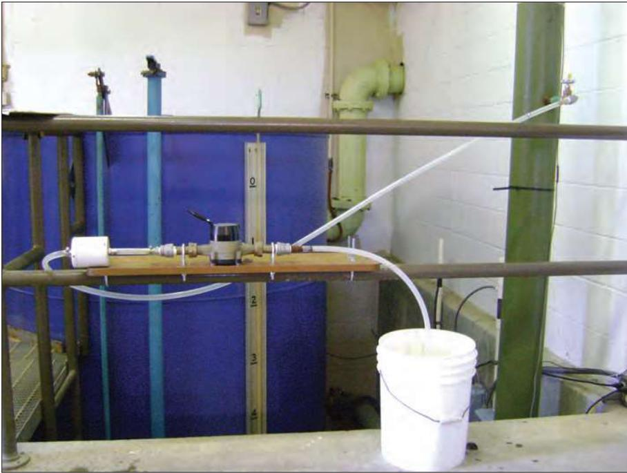
This photo shows a filtering apparatus for *Cryptosporidium* sampling. Note the white filter housing on the left, the water meter, and the filtered water bucket. Also, the vertical, green plant influent line on the right is being sampled. One of the plant's blue filters is in the background.
