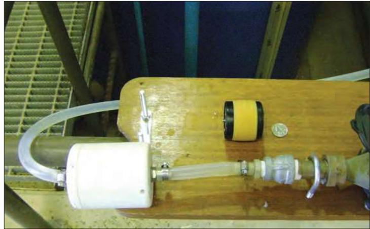
The white filter housing on the left contains a filter to remove Cryptosporidium. A filter with its golden filter media and black ends is also shown nearby.
